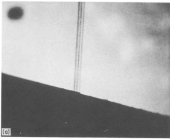
Figure 4 (a) Scratch near edge of microscope slide. (b) Same area as (a) following preheating to 460°C and flashlamp treatment.
